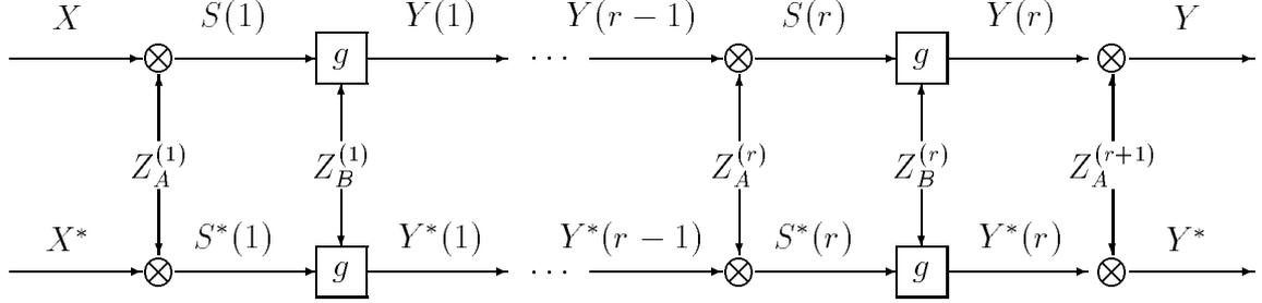
Figure 3: Encrypting a pair of plaintexts with an r-round PES
