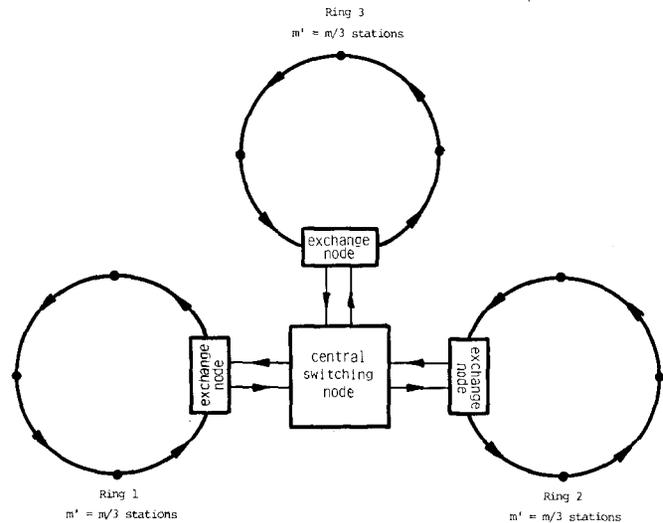
Fig. 5. Communication system consisting of three rings which are interconnected by a star network.
