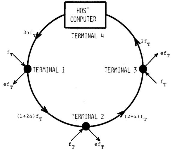
Fig. 3. Ring communication systems with terminal-to-host and host-to-terminal traffic.
