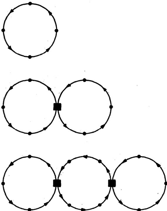
Fig. 1. Examples of communication networks with unique loop-free routing.
