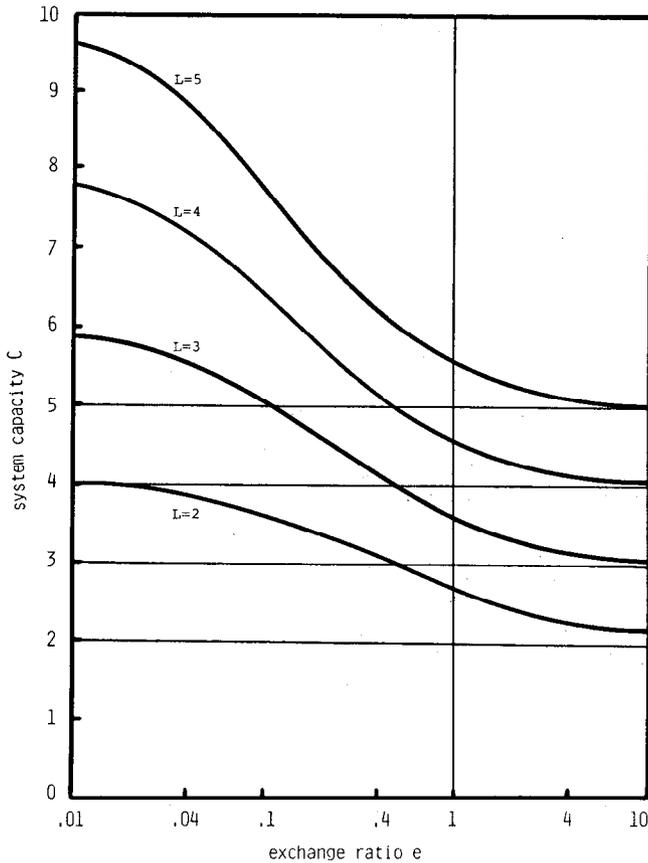
Fig. 6. Capacity of a system with  $m \rightarrow \infty$  stations which are equally split into  $L$  separate rings which are interconnected by a star network (5.3).
