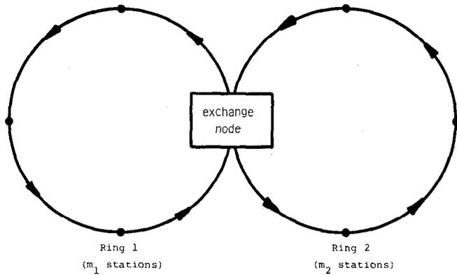
Fig. 4. Communication systems consisting of two rings which are interconnected by an exchange node.
