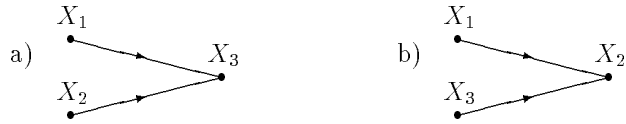
Figure 3: The causality graph of a secret–key cipher (a) in general and (b) when the cipher provides perfect secrecy where X_1 , X_2 and X_3 are the plaintext, secret key and cryptogram, respectively.
