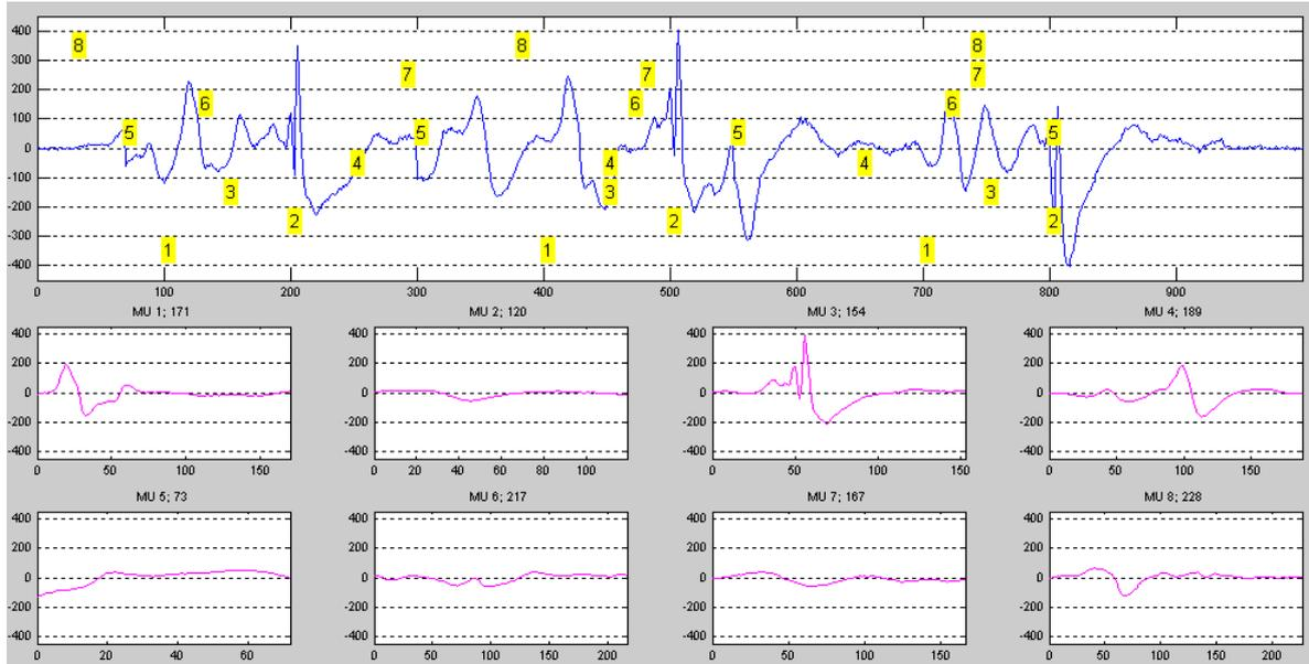
**Fig. 3.** Single-channel EMG signal annotated with the “firing times” of the  $N_{\text{src}} = 8$  sources (top) and the impulse responses of the sources (bottom).
