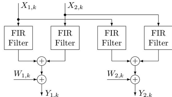
**Fig. 1.** Model of EMG signals for  $N_{\text{src}} = N_{\text{chn}} = 2$ .
