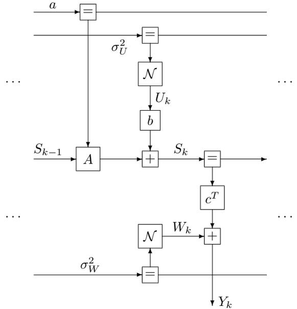
**Fig. 5.** AR parameter estimation: time- $k$  section of the factor graph.
