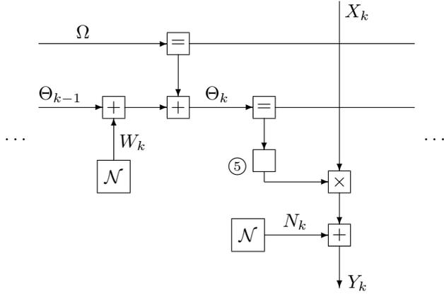
**Fig. 4.** Phase estimation: time- $k$  section of factor graph of (3) and (5).
