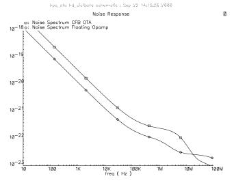
Figure 5: Noise spectra of both circuits.
