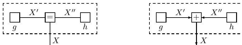
FIG. 8. Summarized function as product (left) and convolution (right) of two local functions.
