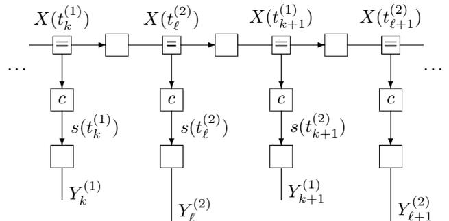
Fig. 1. Factor graph of beamforming as in Section II-A with a state space model of the source/target and with interleaved observations from two sensors.
