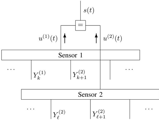
Fig. 2. Beamforming as in Section II-B with two sensors and with a state space model of each sensor. (This figure is not really a factor graph.)
