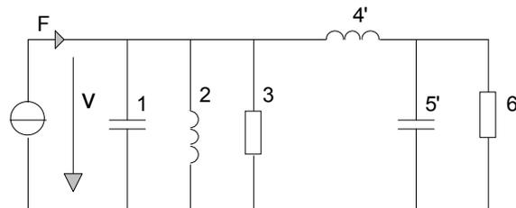
Figure 4: Equivalent electrical network of a simplified violin after dual conversion to get rid of the gyrators.
