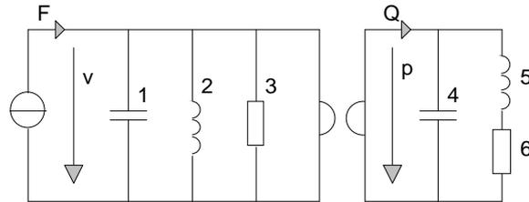
Figure 3: Equivalent electrical network of a simplified violin.
