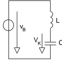
Figure 1: Equivalent electrical network of the mechanical system of the speaker cabin mounted on springs on a heavy ground plate with velocity excitation.
