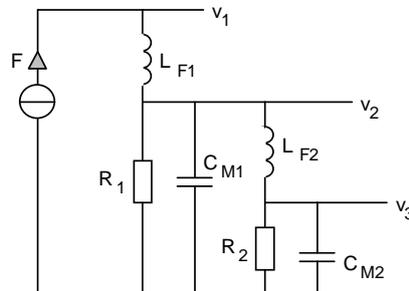
Figure 2: Equivalent network of the system from task 2.
