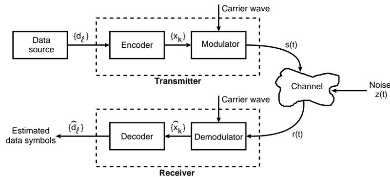
Figure 1: Model of a digital passband transmission system.
