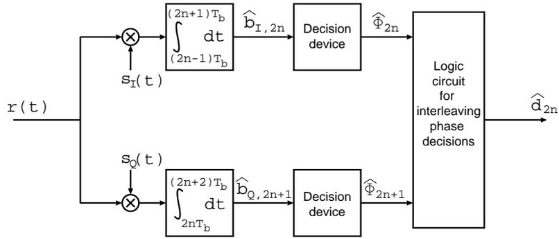
Figure 4: Block diagram of an MSK receiver.
