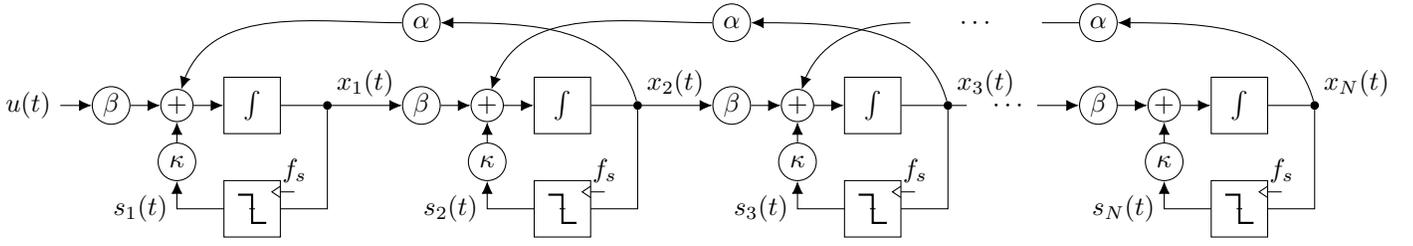
Fig. 1: A  $N$ -th order homogeneous chain-of-integrators (CI) ( $\alpha = 0$ ) and leapfrog (LF) ( $\alpha < 0$ ) control-bounded ADC.
