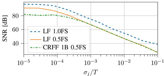
Fig. 4: Simulated SNR vs. normalized RMS jitter ( $\sigma_j/T$ ) for a 3rd order LF and CRFF CTSDM with one bit quantizer (CRFF 1B).
