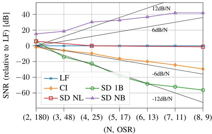
Fig. 2: Simulated and normalized SNR for a LF and CI CBADC compared against CTSDMs with single bit (1B), N-level (NL) and N-bit (NB) quantizers.
