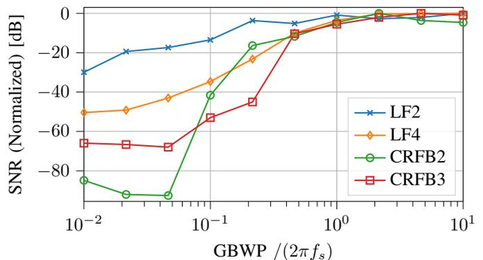
Fig. 5: Simulated normalized SNR vs. normalized amplifier GBWP, for a 2nd and 4th order LF (LF2, LF4) and a 2nd and 3rd order CRFB CTSDM (CRFB2, CRFB3).
