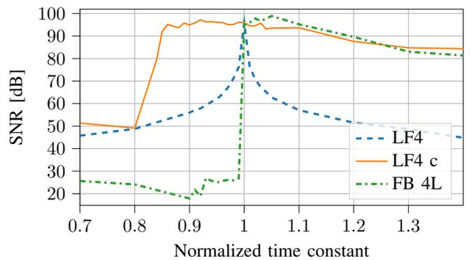
Fig. 3: Simulated SNR vs. normalized time constant for a 4th order CRFB CTSDM with a 4 level (FB 4L) quantizer, and a 4th order LF ADC with (LF4 c) and without (LF4) corrected filter coefficients.
